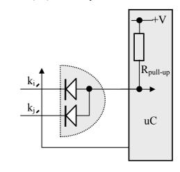
Figure 6. Keypad interface principle for diodes matrix, for one output line, i
