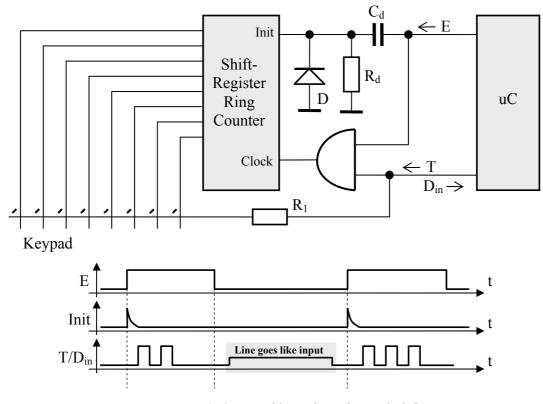
Figure 3. Optimized keypad interface with shift register and bidirectional port lines
