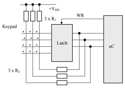
Figure 1. Keypad interface optimized for bidirectional lines port
