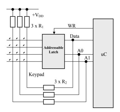
Figure 2. Addressable latch keypad interface for bi-directional lines port
