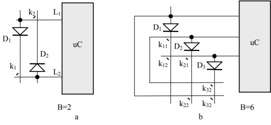
Figure 4. Elementary diodes matrix for bidirectional port lines (one diode per line)
